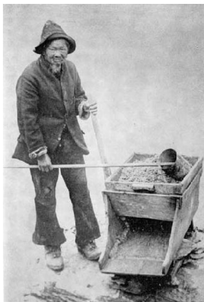
Chinese gold miner feeding a sluicing box
